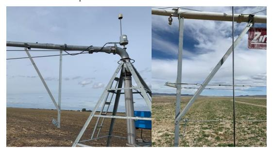
Above Shows the Starter Bracket to the left and Termination Bracket to the right. Below is the Termination bracket face out from the pivot
