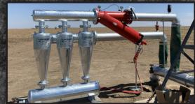
Semi Automatic Brush-away With Sand Separators
